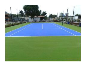
Outdoor highly flexible, acrylic system ideal for tennis, basketball, volleyball, handball, multipurpose courts, as well as any other outdoor sports court. Combination of prefabricated shock-pads and acrylic coating in average total thickness of 6 mm - 14mm.
